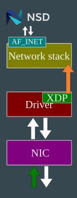
XDP\_TX: send it out of ingress NIC XDP\_DROP: drop the packet **XDP\_PASS**: pass on to network stack
