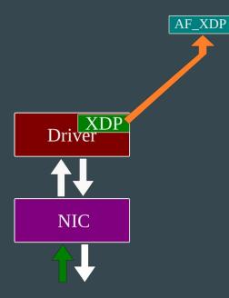
Using the special AF\_XDP socket type one can reach the application while bypassing the entire network stack. (special case of XDP\_REDIRECT)
